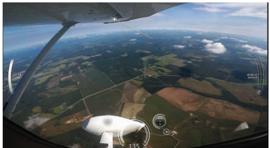
View from a flight camera that records continuous, GPS-linked video of a survey flight.
